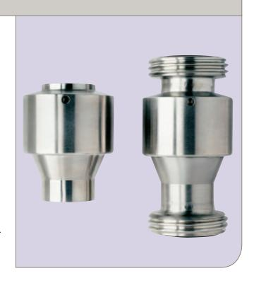
The valve is cleaned in-line during CIP of the vessel. The liquid will close the valve but a special drilling of the valve body ensures cleaning of its seat and the pipe connection because a small amount of liquid flows through.
